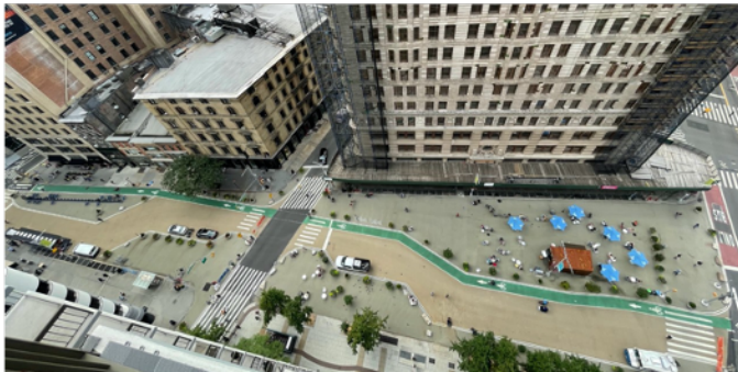
Added pedestrian space and seating amenities with a 5MPH advisory speed limit
